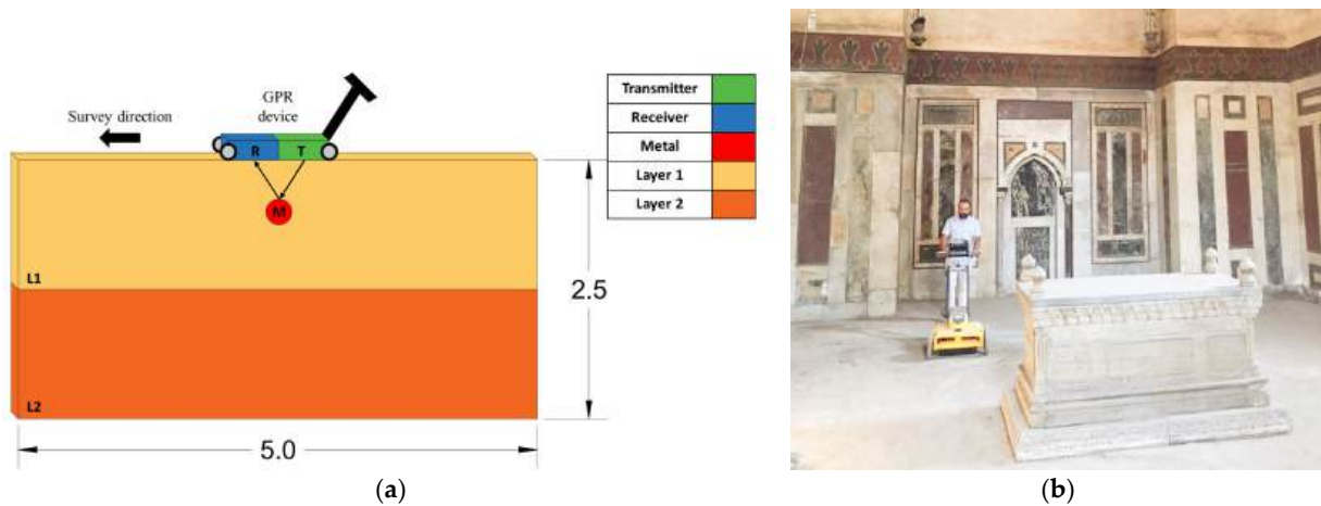
Figure 3. (a) A diagram of the ground-penetrating radar and (b) GPR measurements in Sorghatmesh mosque.
