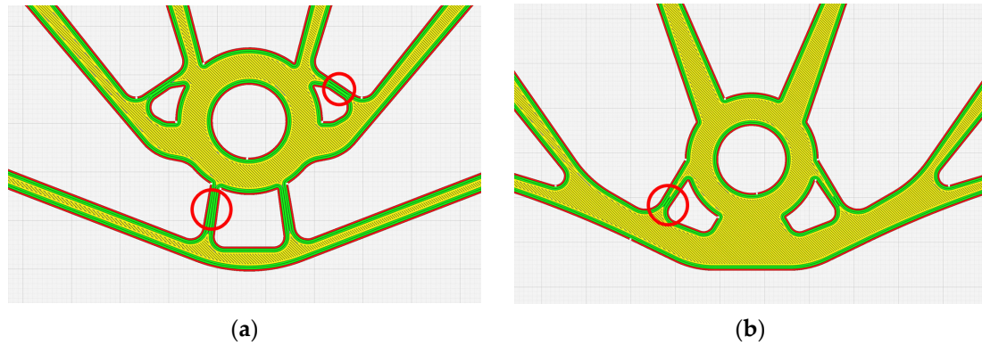
Figure 7. Detail of the critical features for the minimum length constraint. (a) HyperMesh 2023.1 result. (b) MATLAB implementation result. The zones where the minimum length constraint is activated and only six solid perimetral layers are computed are highlighted with red circles.
