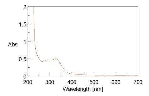
Figure S2. Absorption spectrum of Leaf-Ex.
