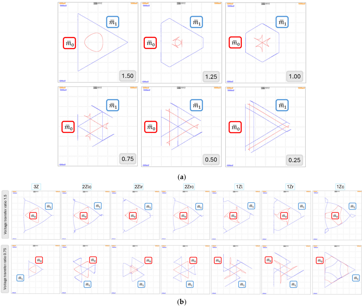
Figure 7. Paths in the complex plane of \bar{m}_1 and \bar{m}_0 for Case 1 (a) and for the conventional SVM strategies (b).
