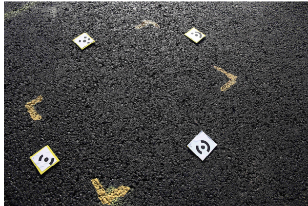
Figure 4. Example of an image acquired by the reflex camera and containing coded targets.
