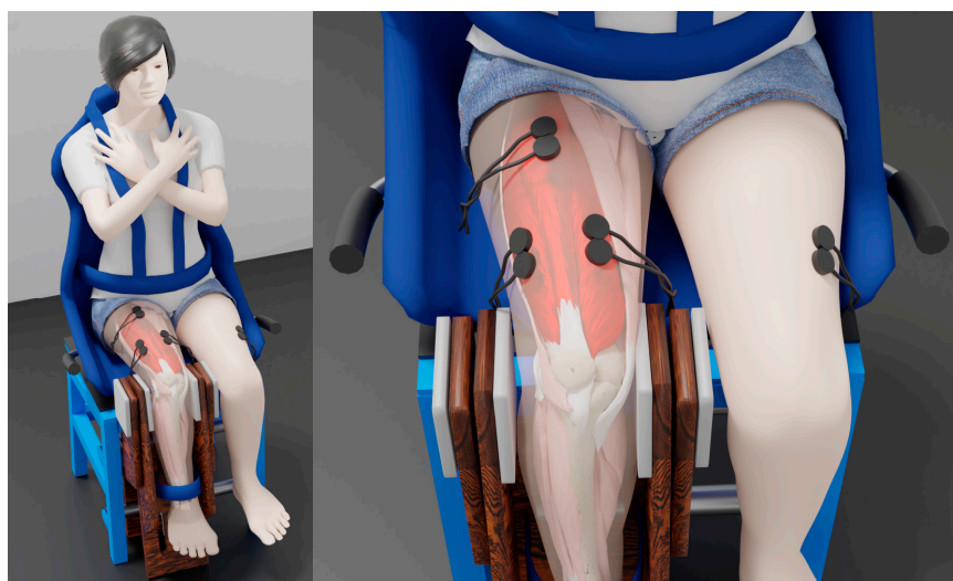
Figure 2. The representation of the experimental setup of the MVIC test of the knee extensors. The subject was placed in a sitting position with the ankle blocked to ensure an isometric position and with each hand on the opposite shoulder throughout the whole test.
