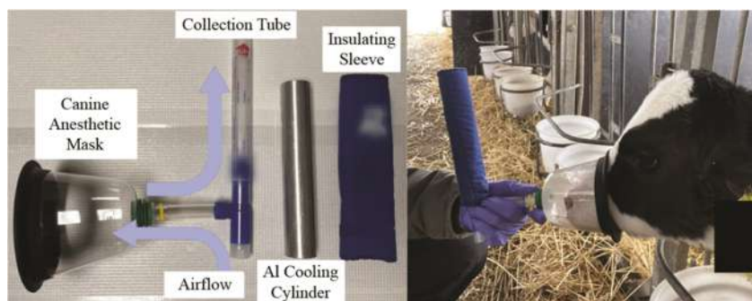
Figure 3. Apparatus used to collect the EBC biospecimens from calves in the field.
