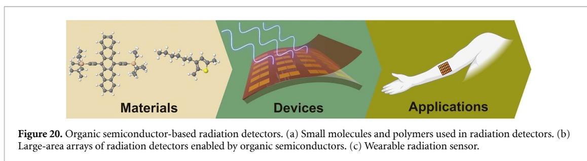
**Figure 20.** Organic semiconductor-based radiation detectors. (a) Small molecules and polymers used in radiation detectors. (b) Large-area arrays of radiation detectors enabled by organic semiconductors. (c) Wearable radiation sensor.
