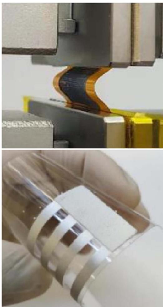
**Figure 43.** Printed chemoresistive gas sensor undergoing repeated automated bending tests for studying its reliability. Au Interdigitated electrodes are printed on polyimide by inkjet and the gas sensitive film consists of air-brushed polypyrrole nanoparticles supported on graphene flakes (top). Printed piezoelectric energy harvester on polyethylene. The piezoelectric film consists of polyvinyl acetate + poly(3,4-ethylenedioxythiophene) + ZnO.
