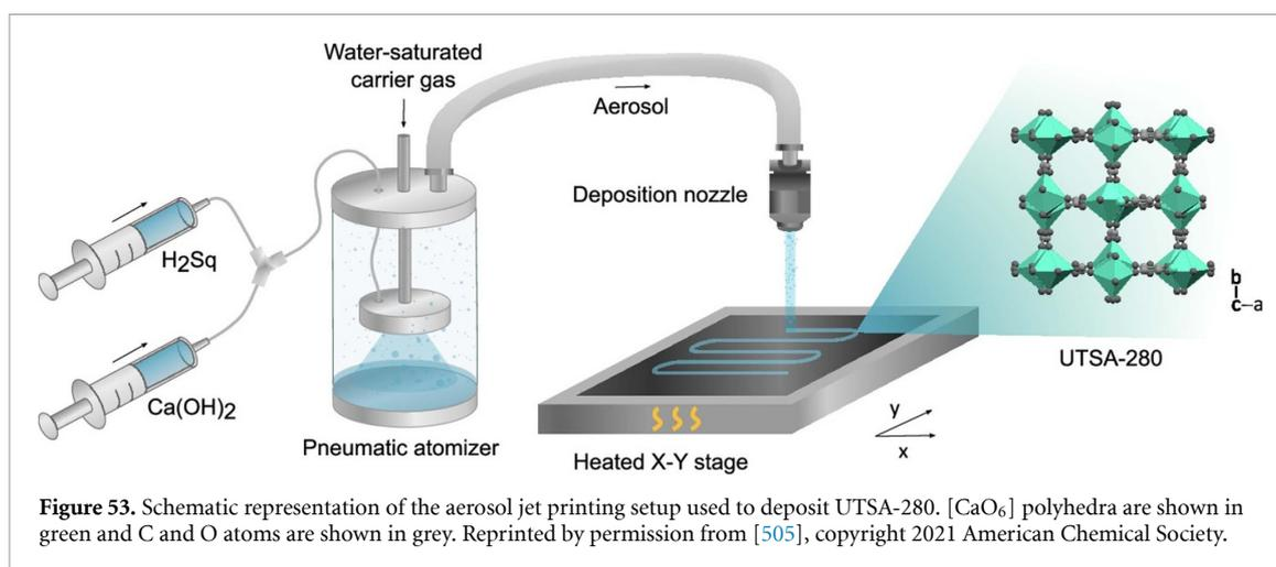
**Figure 53.** Schematic representation of the aerosol jet printing setup used to deposit UTSA-280.  $[\text{CaO}_6]$  polyhedra are shown in green and C and O atoms are shown in grey. Reprinted by permission from [505], copyright 2021 American Chemical Society.
