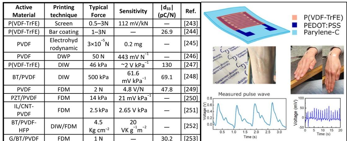
**Figure 25.** Left: typical parameters of printed PVDF-based pressure sensors. Right: Example of a printed transparent pressure sensor for bio-signal monitoring based on P(VDF-TrFE). Reproduced from [255]. CC BY 4.0. Copyright © 2021 The Authors. Published by American Chemical Society. This publication is licensed.
