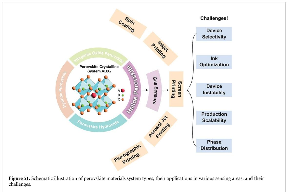
**Figure 51.** Schematic illustration of perovskite materials system types, their applications in various sensing areas, and their challenges.
