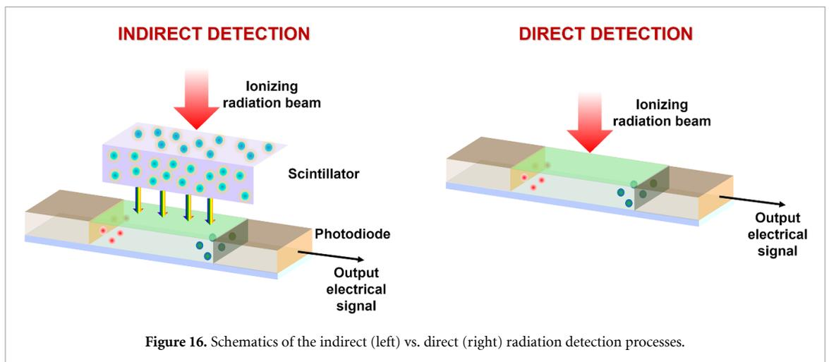
Figure 16. Schematics of the indirect (left) vs. direct (right) radiation detection processes.
