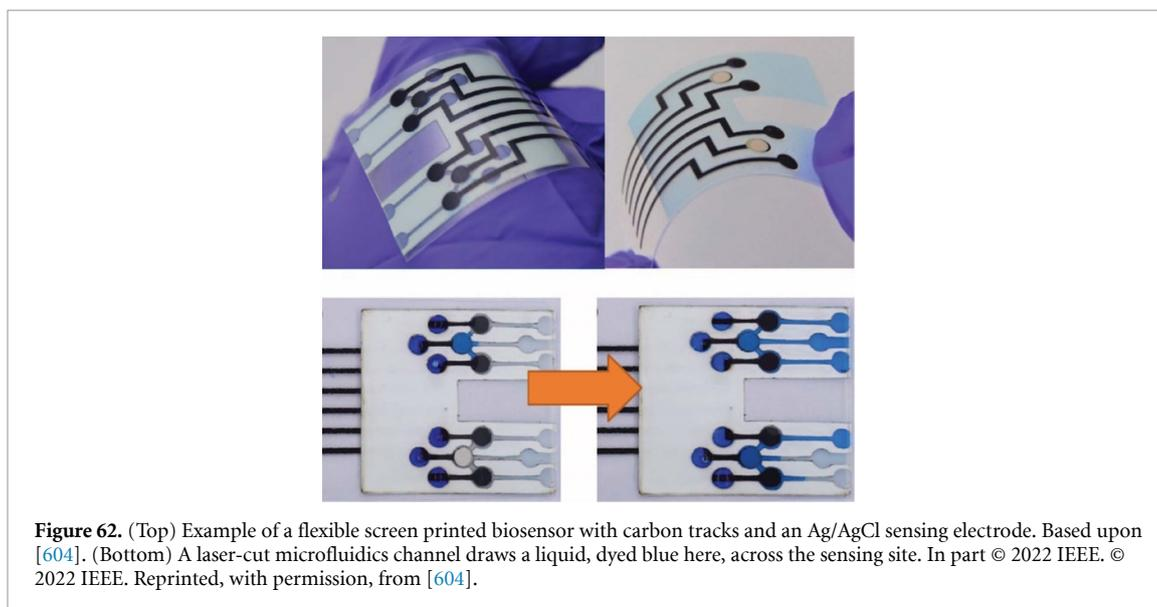
**Figure 62.** (Top) Example of a flexible screen printed biosensor with carbon tracks and an Ag/AgCl sensing electrode. Based upon [604]. (Bottom) A laser-cut microfluidics channel draws a liquid, dyed blue here, across the sensing site. In part © 2022 IEEE. © 2022 IEEE. Reprinted, with permission, from [604].
