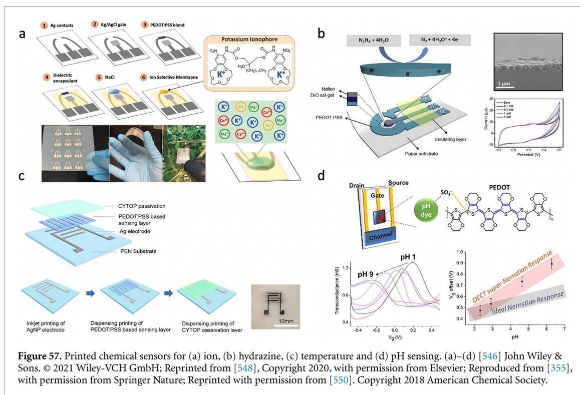
**Figure 57.** Printed chemical sensors for (a) ion, (b) hydrazine, (c) temperature and (d) pH sensing. (a)–(d) [546] John Wiley & Sons. © 2021 Wiley-VCH GmbH; Reprinted from [548], Copyright 2020, with permission from Elsevier; Reproduced from [355], with permission from Springer Nature; Reprinted with permission from [550]. Copyright 2018 American Chemical Society.
