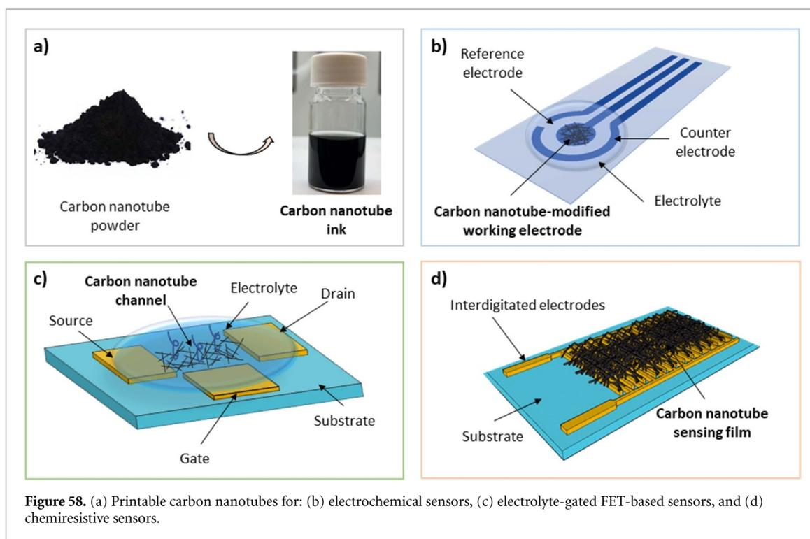
**Figure 58.** (a) Printable carbon nanotubes for: (b) electrochemical sensors, (c) electrolyte-gated FET-based sensors, and (d) chemiresistive sensors.
