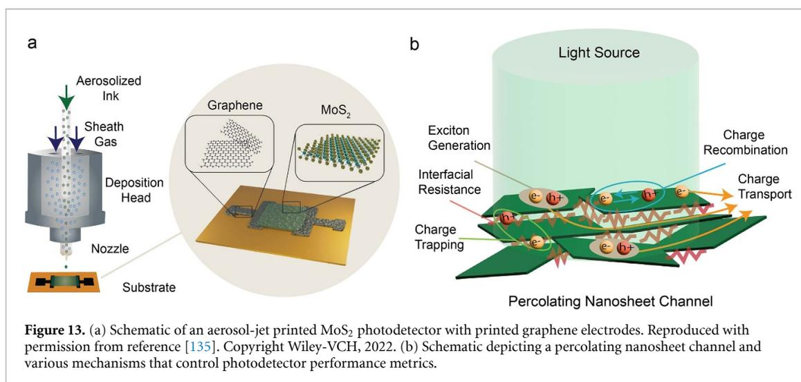
**Figure 13.** (a) Schematic of an aerosol-jet printed MoS<sub>2</sub> photodetector with printed graphene electrodes. Reproduced with permission from reference [135]. Copyright Wiley-VCH, 2022. (b) Schematic depicting a percolating nanosheet channel and various mechanisms that control photodetector performance metrics.
