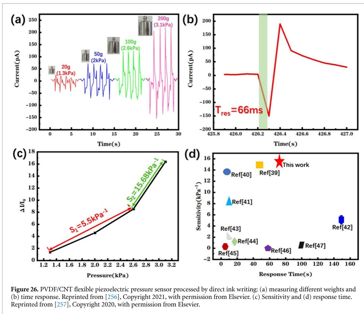
**Figure 26.** PVDF/CNT flexible piezoelectric pressure sensor processed by direct ink writing: (a) measuring different weights and (b) time response. Reprinted from [256], Copyright 2021, with permission from Elsevier. (c) Sensitivity and (d) response time. Reprinted from [257], Copyright 2020, with permission from Elsevier.
