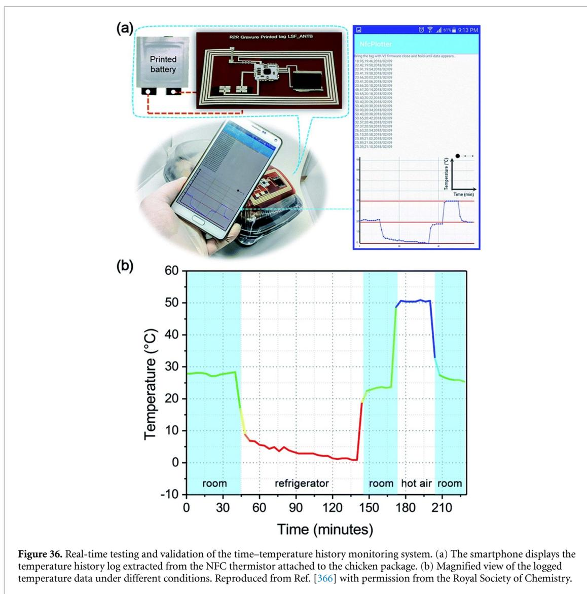
**Figure 36.** Real-time testing and validation of the time–temperature history monitoring system. (a) The smartphone displays the temperature history log extracted from the NFC thermistor attached to the chicken package. (b) Magnified view of the logged temperature data under different conditions. Reproduced from Ref. [366] with permission from the Royal Society of Chemistry.
