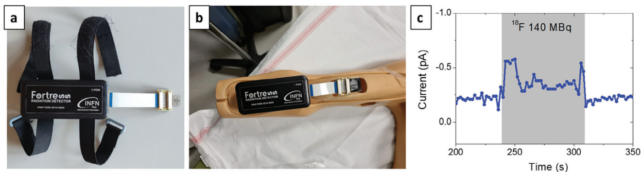
Figure 6. a) Wireless and wearable electronic readout system, connected to the detector through a flat cable. b) Detector system worn by the arm of an anthropomorphic phantom. c) Signal recorded and transmitted via WiFi, monitoring the gamma rays emitted by the flow of ^{18}\text{F} radiotracer inside the plastic tubing of the phantom mimicking the vein. The signal was collected with a detector bias voltage of 2 V.
