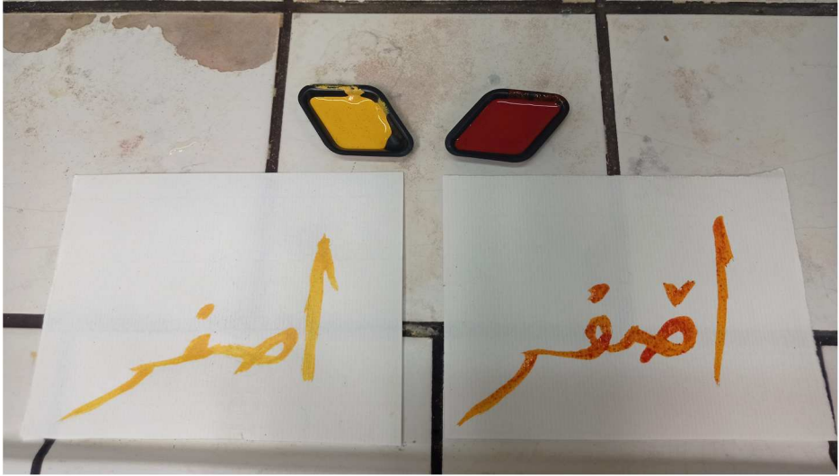
FIGURE 1 Writing samples realised with primary yellow from pure orpiment (left) and compound yellow from lead white and saffron (right). Photo: L. Raggetti.
