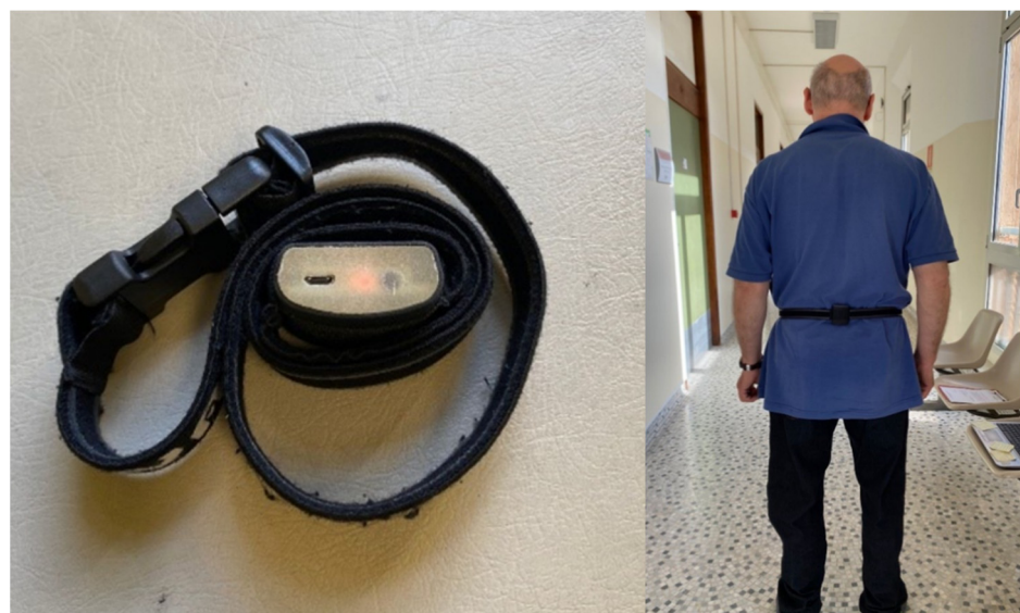
Figure 1. Wiva ® MOB device in use for kinematics analysis in this study (left); example of sensor positioning on a participant (right).
