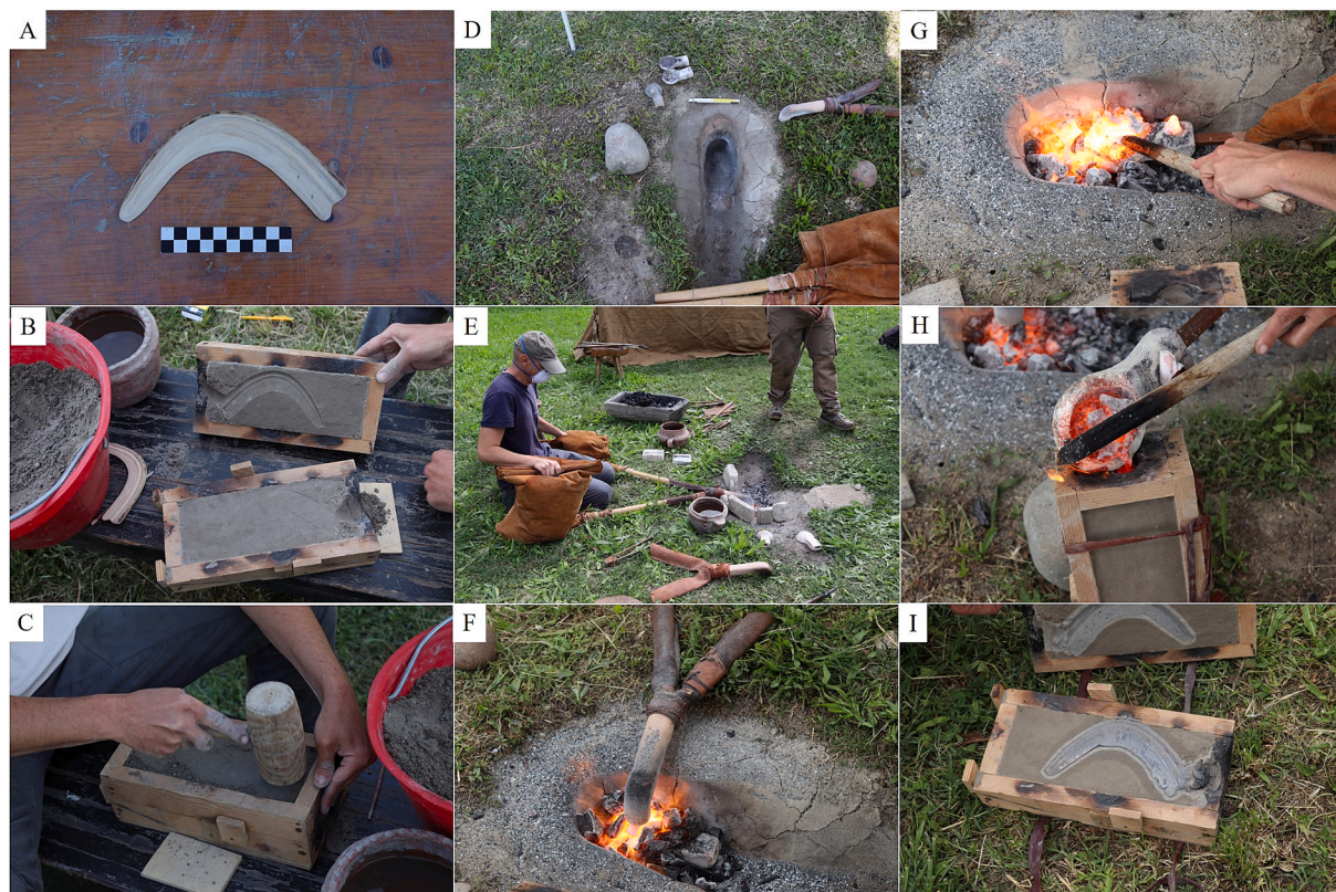
Fig. 2. Examples of sickle replicas. a. sickle replicas in wood; b-c. production and use of the sand mould. d-e; preparation of the casting pit feeding the coals with air blown by tuyeres; f-g. melting of copper and tin inside a crucible; h. pouring the obtained bronze alloy into the sand mould; i. removing the replica from the mould.
