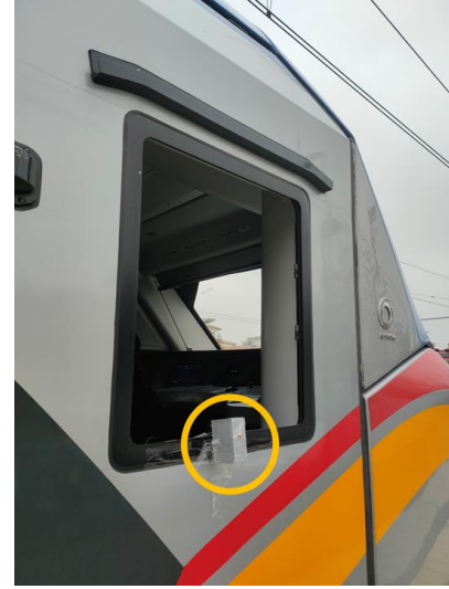
Fig. 12. Positioning of the 2.45 GHz antenna module with PLA case outside the cockpit.
