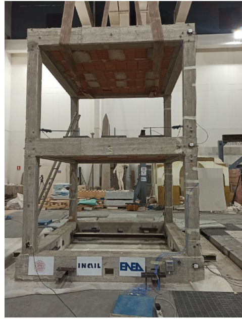
Fig. 1: MAC4PRO monitored concrete structure.
