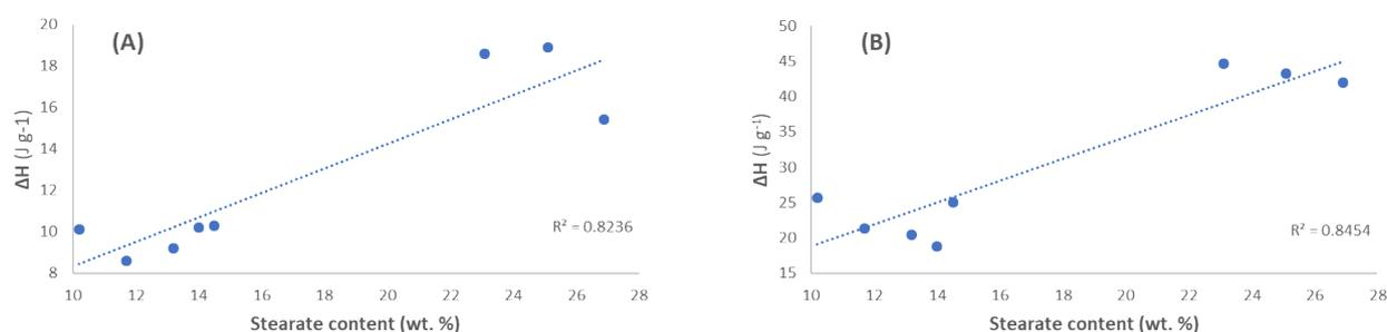
**Figure S9.** Relationship between the dehydration enthalpy (A) and the crystalline-to-smectic transition enthalpy (B) for the Ca stearate layer adsorbed on the CaCO<sub>3</sub> particles surface versus the adsorbed percentage of stearate.
