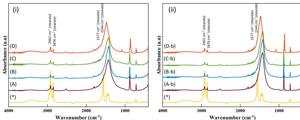
**Figure S10.** FTIR spectra of unbleached and bleached powders (A) geogenic  $\text{CaCO}_3$ , (B) oyster shells, (C) scallop shells and (D) clam shells coated using a 40 mM stearate solution. (i) unbleached  $\text{CaCO}_3$  samples. (ii) bleached  $\text{CaCO}_3$  samples. (\*) Sodium stearate FTIR spectrum.
