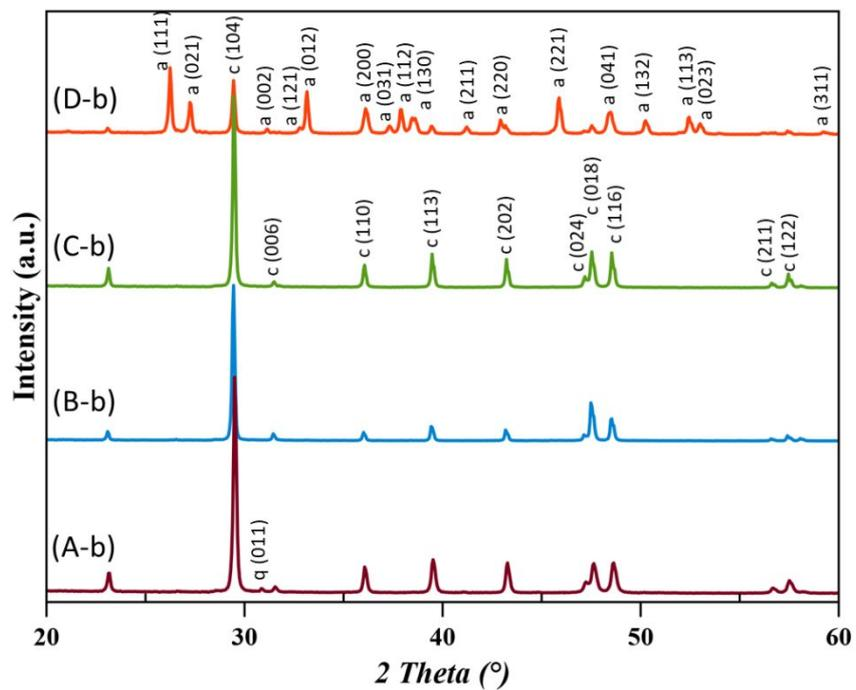
**Figure S3.** X-ray powder diffraction patterns of bleached geogenic  $\text{CaCO}_3$  (A-b), oyster shell (B-b), scallop shell (C-b) and clam shell powder (D-b). The diffraction patterns were indexed accordingly to the PDF 00-005-0586 for calcite (c), PDF 00-005-0453 for aragonite (a) and PDF 01-080-2148 for quartz (q).
