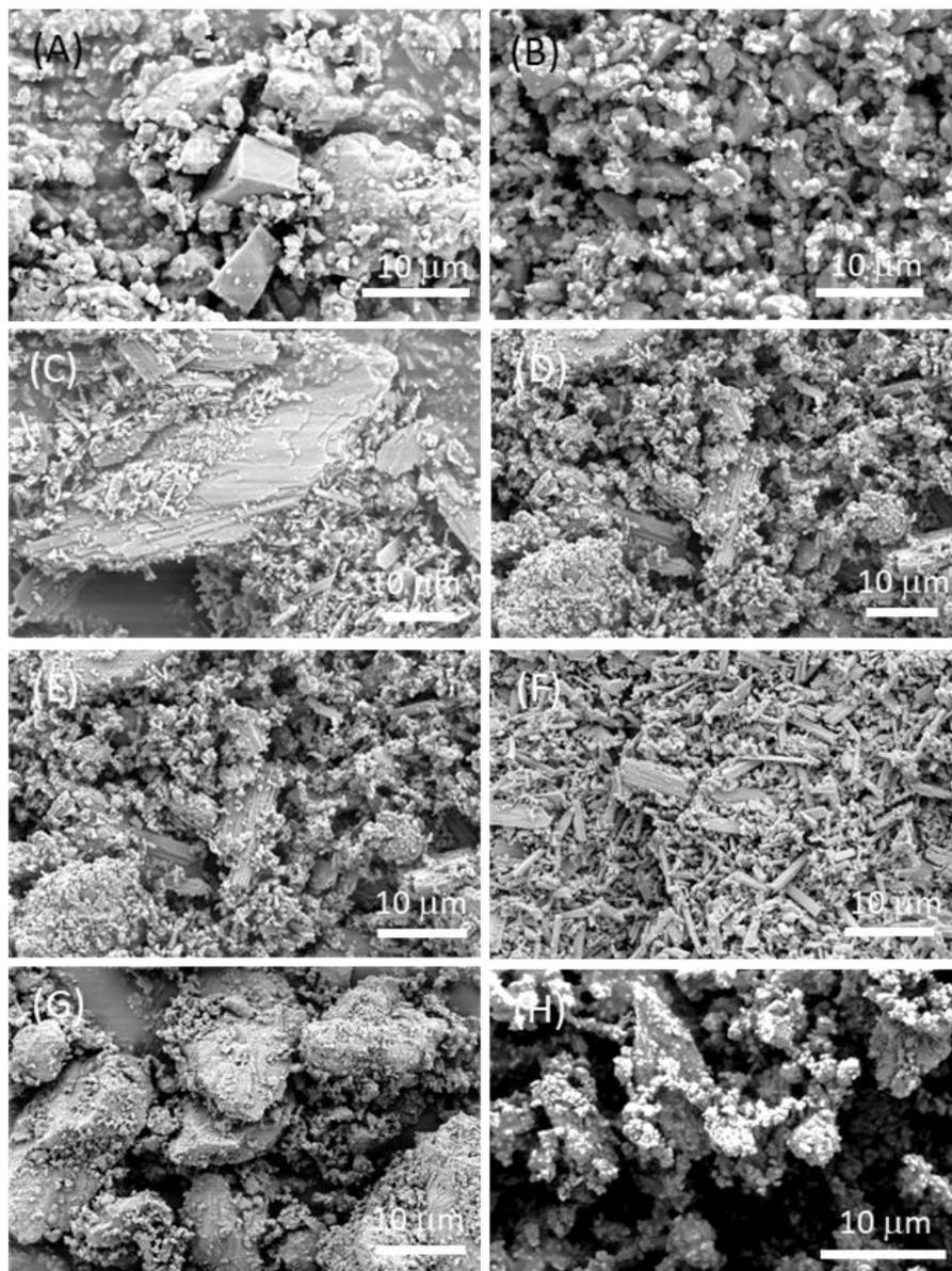
**Figure S4.** Low magnification SEM images of unbleached (A, C, E and G) and bleached (B, D, F and H) powders from geogenic calcite (A, B), oyster shells (C, D), scallop shells (E, F) and clam shells (G, H). These images are representative of the entire population of particles.
