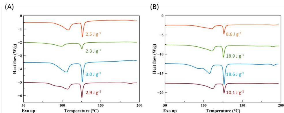
**Figure S7.** DSC profiles of powder of geogenic CaCO<sub>3</sub> (red), oyster shells (blue), scallop shell (green) and clam shell (orange) coated with 40 mM (A) and 400 mM (B) aqueous sodium stearate solutions.
