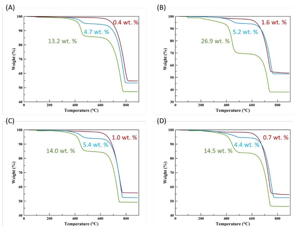
**Figure S6.** TGA profiles of bleached powder of geogenic CaCO<sub>3</sub> (A), oyster shells (B), scallop shells (C) and clam shells (D) (red) and corresponding coated powder with 40 mM (blue) and 400 mM aqueous sodium stearate (green) solutions.
