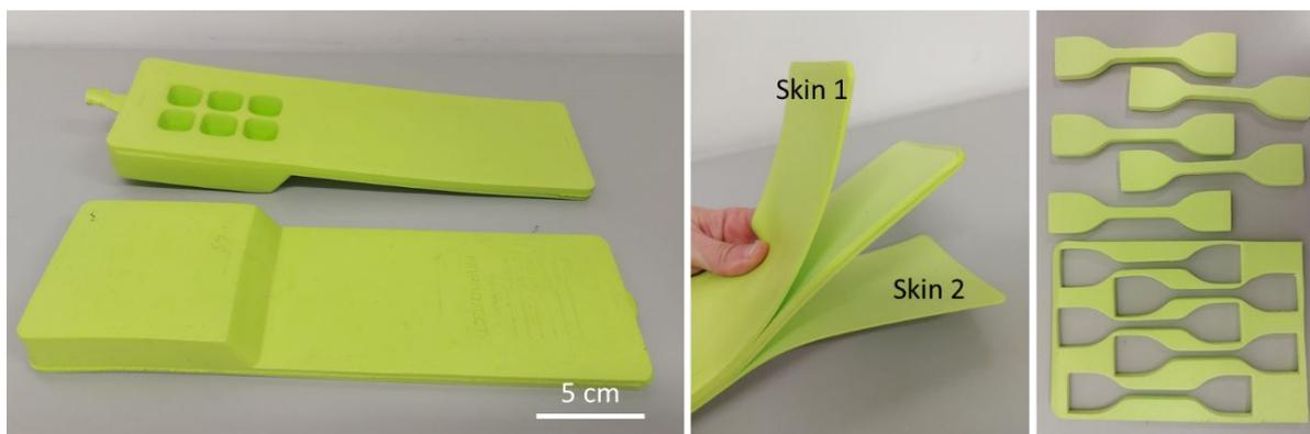
**Figure S1.** Polymeric compound specimen preparation for mechanical and aesthetic evaluations.
