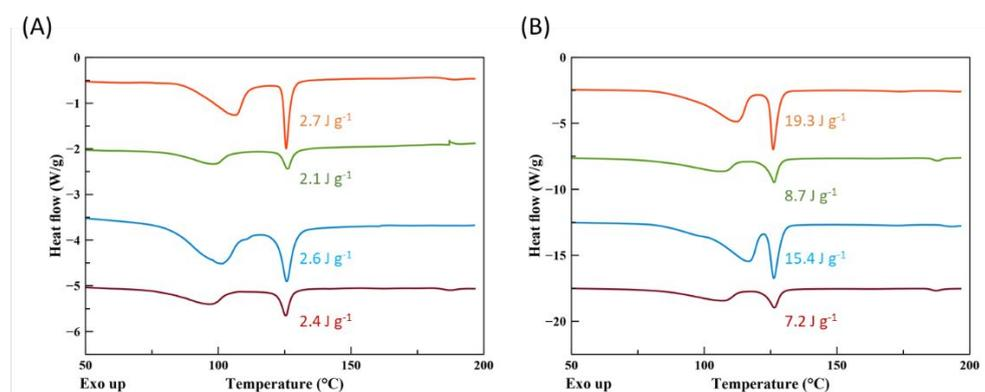
**Figure S8.** DSC profiles of powder of bleached geogenic CaCO<sub>3</sub> (red), oyster shells (blue), scallop shells (green) and clam shells (orange) coated with 40 mM (A) and 400 mM (B) aqueous sodium stearate solutions.
