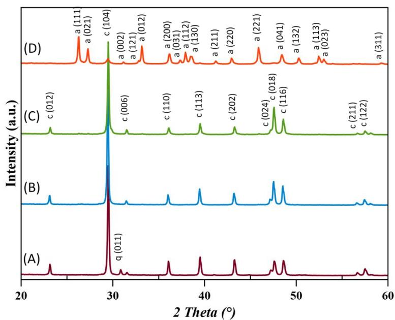
**Figure S2.** X-ray powder diffraction patterns of geogenic  $\text{CaCO}_3$  (A), oyster shell (B), scallop shell (C) and clam shell powder (D). The diffraction patterns were indexed accordingly to the PDF 00-005-0586 for calcite (c), PDF 00-005-0453 for aragonite (a) and PDF 01-080-2148 for quartz (q).
