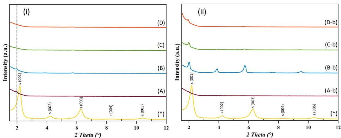
**Figure S11.** X-ray powder diffraction patterns of unbleached and bleached powders (A) geogenic  $\text{CaCO}_3$ , (B) oyster shells, (C) scallop shells and (D) clam shells coated using a 40 mM stearate solution. (i) unbleached  $\text{CaCO}_3$  samples. (ii) bleached  $\text{CaCO}_3$  samples. (\*) Sodium stearate X-ray powder diffraction pattern.
