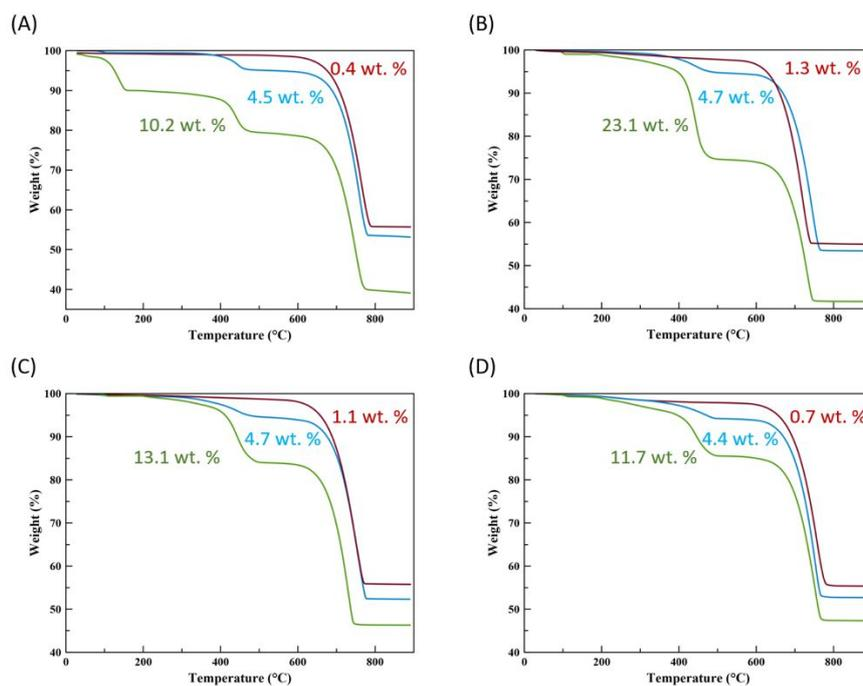
**Figure S5.** TGA profiles of powder of geogenic CaCO<sub>3</sub> (A), oyster shells (B), scallop shells (C) and clam shells (D) (red) and corresponding coated powder with 40 mM (blue) and 400 mM aqueous sodium stearate (green) solutions.
