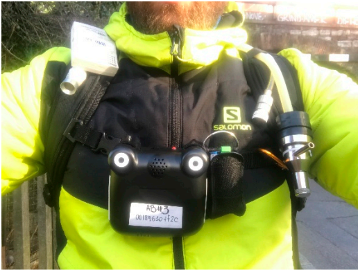
Figure S2. Setup of the instruments placed in a backpack. Inlets were placed in the breathing zone of the operator.
