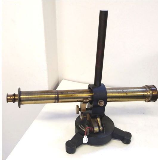
Fig. 5. The reflector Poggendorff scale of the Physics Collection of Bologna. Credit: University Museum Network, University of Bologna
