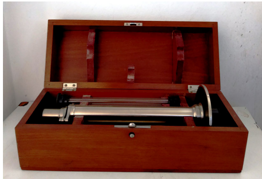
Fig. 3. One the optical tubes in the Physics Collection of Bologna, captioned as “Reflector Poggendorff Scale” but identified instead as a saccharimeter. Credit: University Museum Network, University of Bologna
