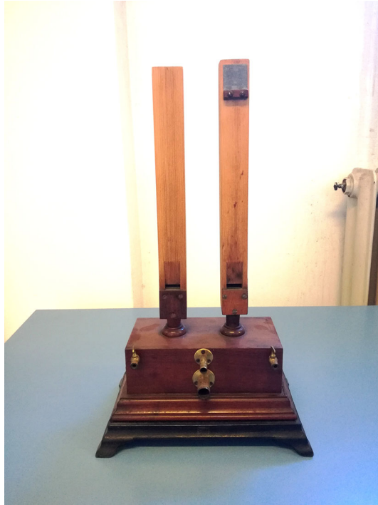
Fig. 7. Incomplete apparatus for the comparison of the vibrations of two air columns of the Physics Collection of Bologna. Credit: University Museum Network, University of Bologna
