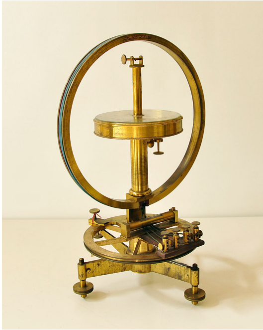
Fig. 2. One of the two compasses of the sines and of the tangents of the Physics Collection of Bologna. The instrument bears the signature of Heinrich Ruhmkorff. Credit: University Museum Network, University of Bologna
