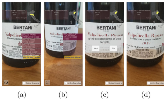
Fig. 3 AR interface: a, b wrong and correct suggestions, c correct confirmation, d after the confirmed identification, the scan stops
