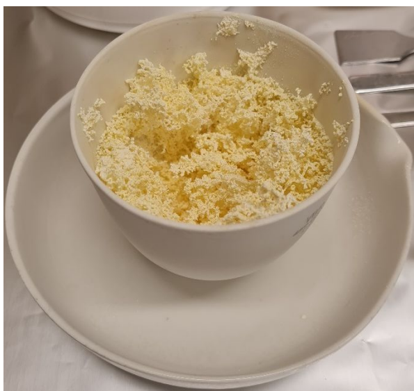
Figure S2. Optical image of \text{In}_2\text{O}_3 prepared by urea combustion method.
