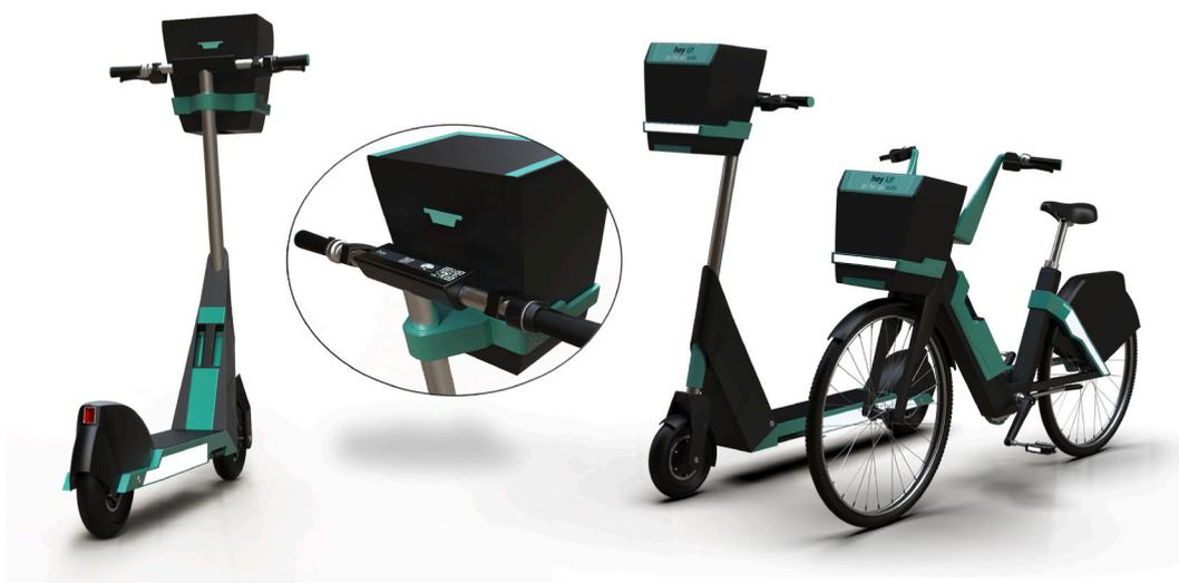
Fig. 7. Sanitizer mounted on some vehicles (scooter and bicycle).
