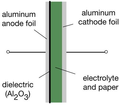
Fig. 1: Basic structure of an aluminum electrolytic capacitor.
