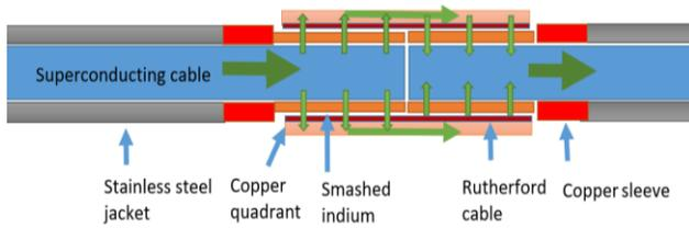
Fig. 7. Current transfer schematic in the coaxial joint
