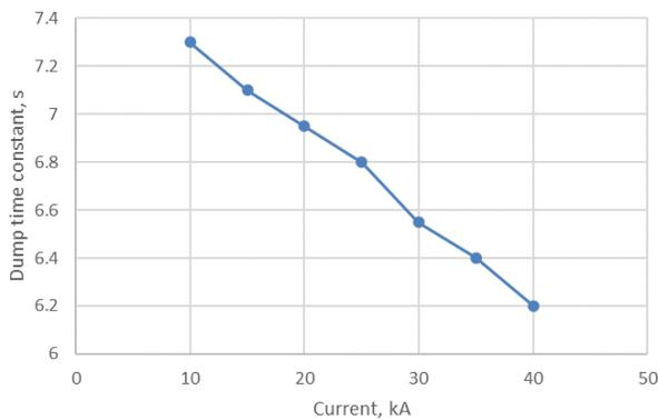
Fig. 8. Decay time of dumps vs initial current
