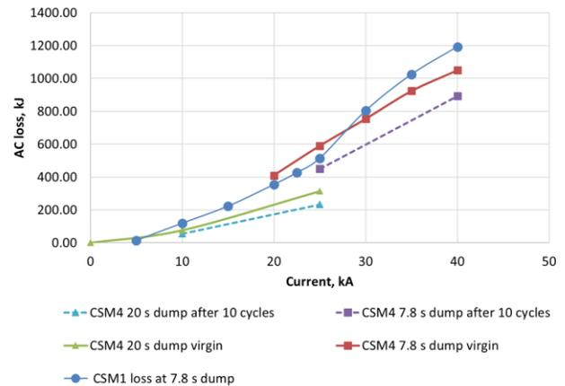
Fig. 9. AC losses in CSM4 by isochoric method
