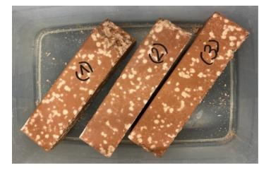
**Figure 5.** Image of three different mixes of C2 specimens (with R aggregates) with the presence of white stains a few days after the demolding procedure.
