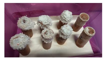
Figure 6. Efflorescence in the cylinders tested for determination of water absorption by capillary.
