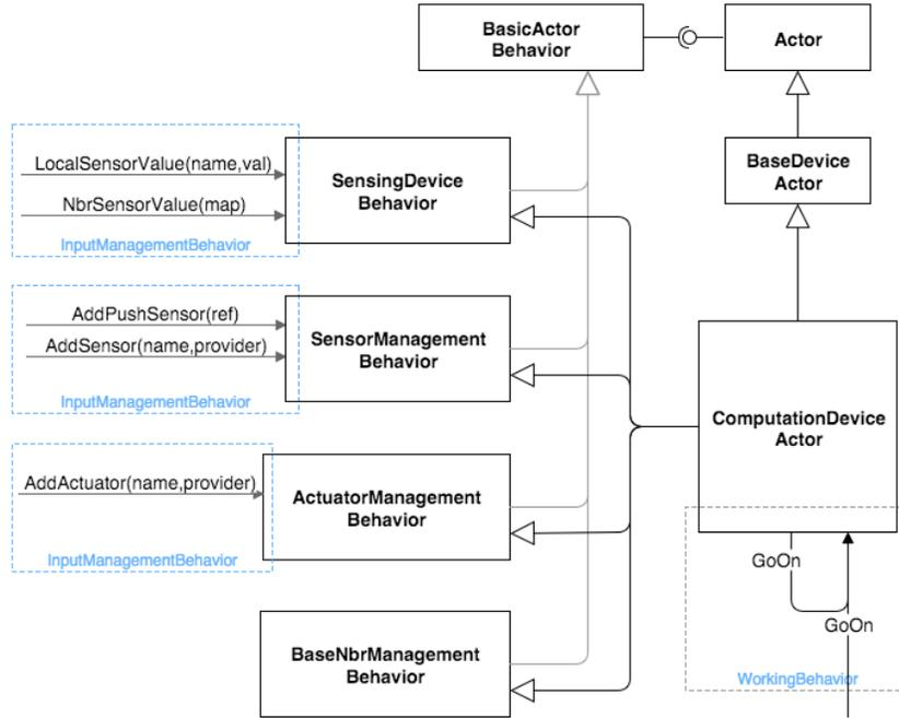
Fig. 4. Structure and interface of device actors.
