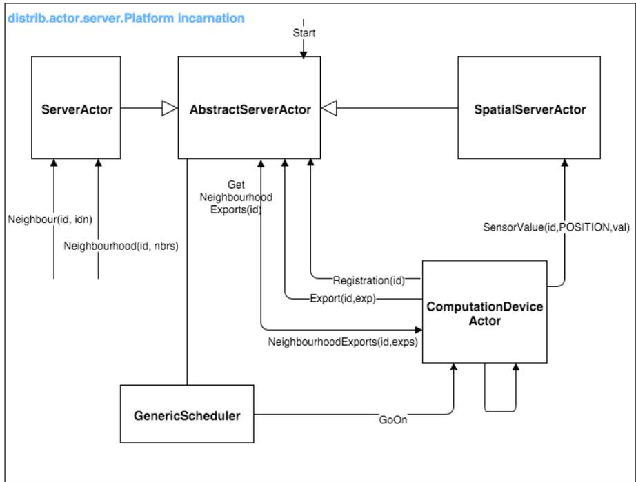
Fig. 5. Key elements and relationships in a server-based actor platform.
