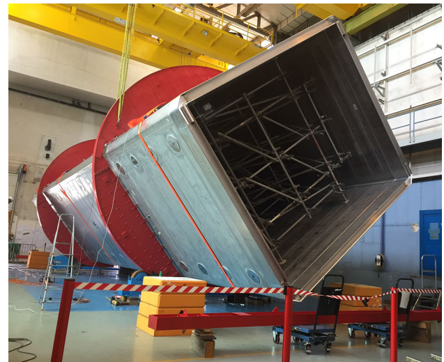
Fig. 2 One of the two new ICARUS cryostats during its assembly at a CERN workshop
