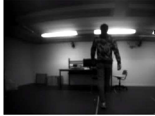
(a) Grayscale QVGA image captured by the AI-Deck . A person is walking at approximately 1.7 meter from the nano-drone. Note that the Himax HM01B0 camera is saturating due to the indoor lighting
