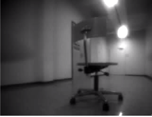
(a) Grayscale QVGA image captured by the AI-Deck . A chair is placed at approximately 55 cm from the nano-drone
