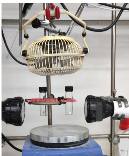
Figure S1. Reaction setup using EvoluChem lamps emitting at 405 nm
