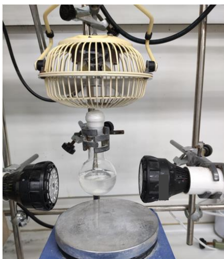
Figure S2. Setup for the gram-scale experiment using two EvoluChem lamps emitting at 405 nm.
