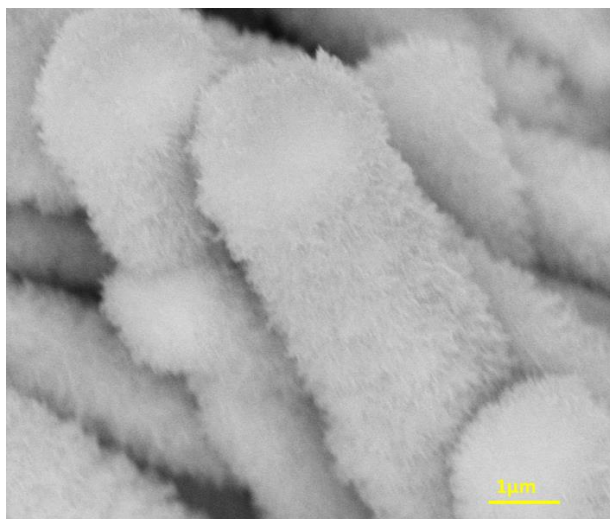
Figure S 6 . SEM images of NiMoO 4 /MoS 2 after stability test.
