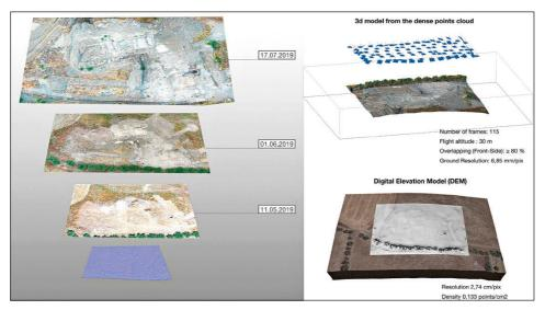
Fig. 3 – Sequence of flight missions and restitution of the Digital Elevation Model.
