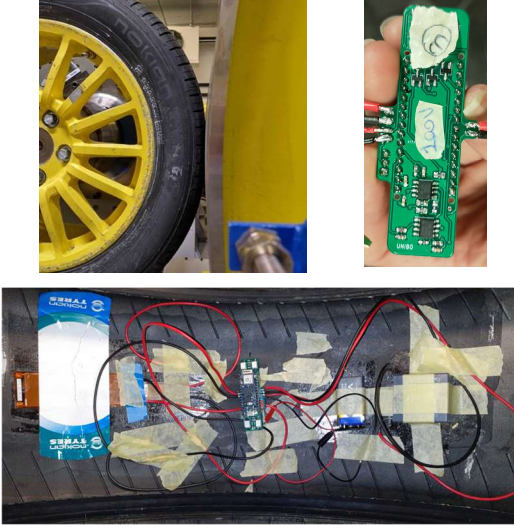
Fig. 6. The drum test machine used for experiments (top left); a picture of the PCB of the telemetry system (top right); an example of experimental setup.
