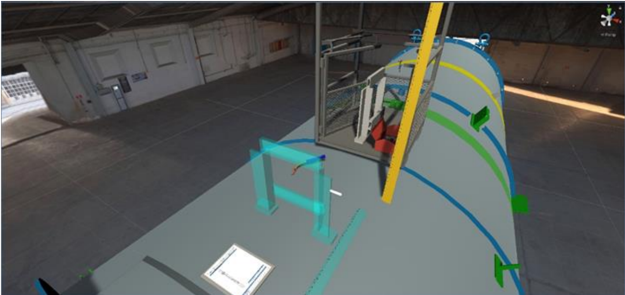
Fig. 2: VR simulation of tracing of auxiliary elements to be subsequently welded on the cans.
