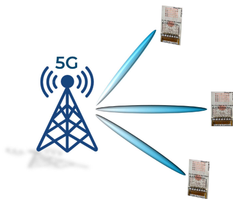
FIGURE 20. Schematic showing a 5G/mm-wave base station steering its beam to energize and communicate with IoT devices.
