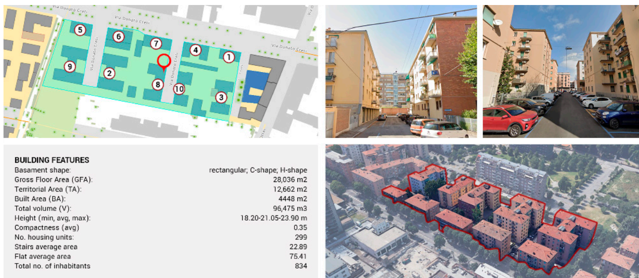
Figure 8. Case study FID 273: positioning, geometric, and constructive characterisation of buildings. © Authors' graphical elaboration.
