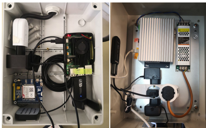
Figure 5: The implemented Wi-Fi end-point sniffer (left) and Vehicular system (right).
