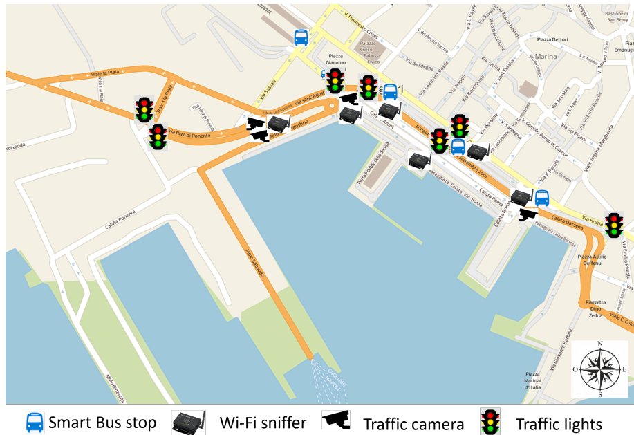
Figure 4: The Roma Street and New York 11th September” Promenade scenario equipped with Wi-Fi sniffer and Traffic camera.
