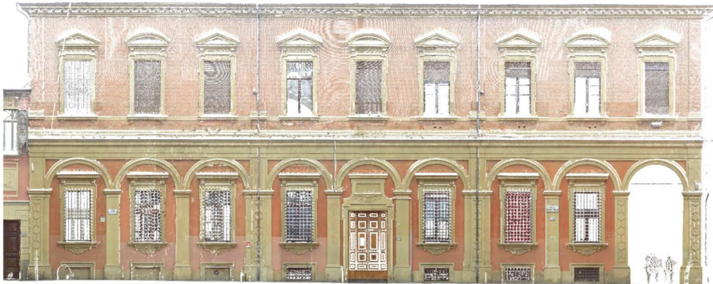
FIGURE 7 - Palazzo Poggi elevation, laser scanner survey
