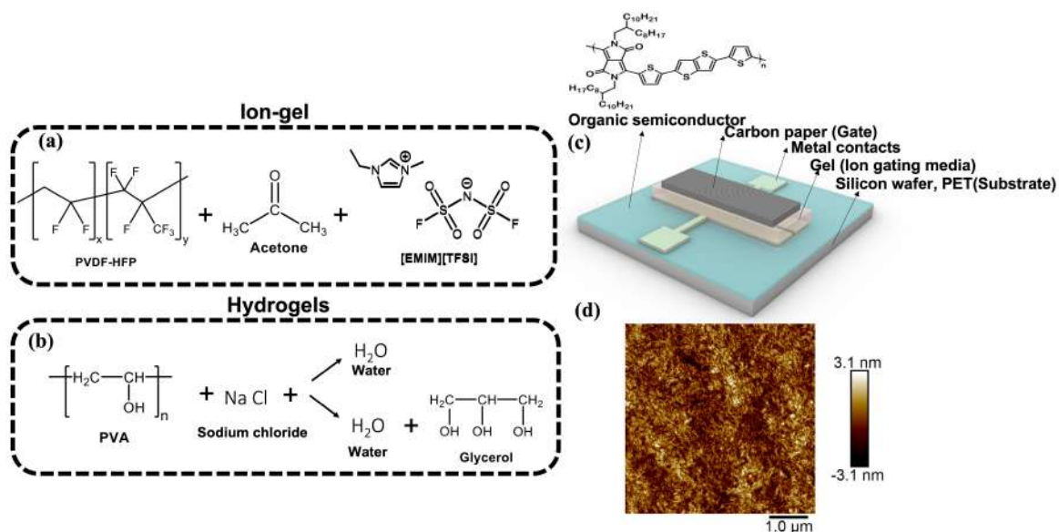
Figure 1. Molecular structures of the materials used for iongels (a) and hydrogels (b), scheme of device and molecular structure of the organic semiconductor (DPP-DTT) (c), AFM image of spin-coated DPP-DTT film on Si/SiO 2 substrate (d).
