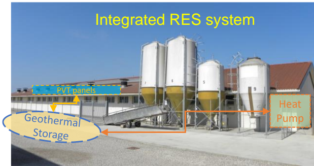
Figure 3. Scheme of the integrated RES system.
