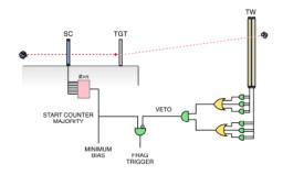
Figure 2: Sketch of a fragmentation event (drawing not in scale). The fragment is generated on the target and, in this example, hit the Tof-Wall out from the center.
