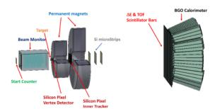
Figure 1: Sketch of the FOOT detector. The ion beam goes from left to right, the primary ion is detected by the Start Counter scintillation foil and then tracked by the Beam Monitor drift chamber, downstream the target fragments are tracked by silicon pixel and strip detectors and finally inping the Tof-Wall for the time of flight and dEdX measurements and the calorimeter.
