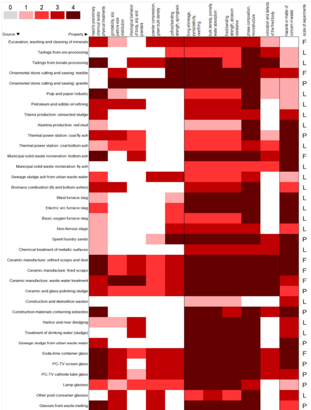
Figure 5. Matrix of technological information available for waste recycling in ceramic tiles. Color codes represent: full characterization by multiple sources (4); full characterization by a single source or partial characterization by multiple sources (3); partial characterization by a single source and/or contradictory data by multiple sources (2); characterization not relevant for ceramic tiles (1); no data (0). Experimentation carried out up to: L) laboratory scale; P) pilot line or lab scale approaching industrial conditions; F) full scale or industrial plant.
