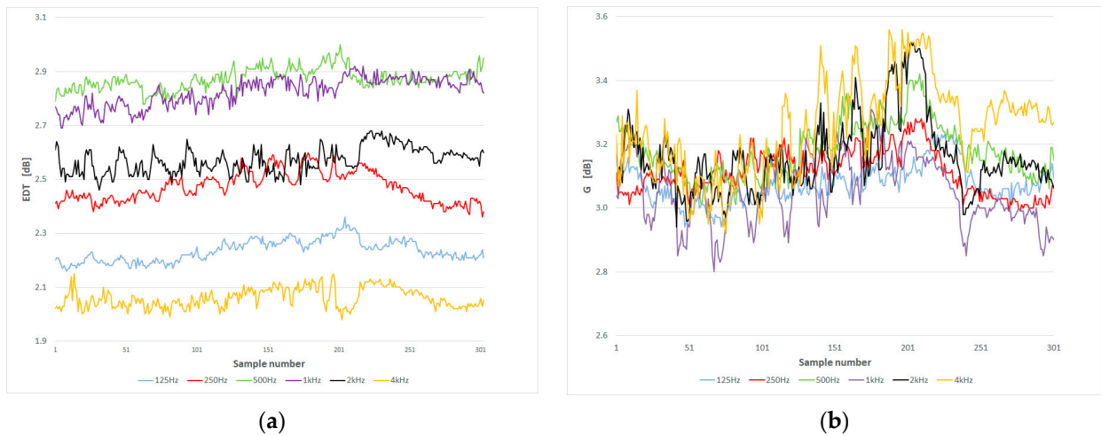
Figure 6. Early decay time (EDT) trends (a), strength (G) trends (b), similar parametric trends.
