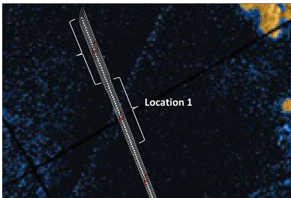
Fig. 7 Detail of the effective area size for a portion of Ligeia Mare close to location 1 from Fig. 6. A trail of white markers draws a specular point track with 2.048 s of resolution. The white ellipses are the respective effective areas along the track. The red markers coincide with the yellow dots from the specular point track of Fig. 6, resolution equal to the processing count time: 61.44 s. Each value of rms slope or dielectric constant, which is associated to a reflecting region centered at each red dot, averages what happens in the set of effective areas grouped by a curly bracket
