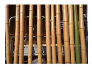
Figure 2. Drying of an untreated green culm and several treated ones.
