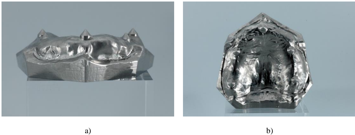
Fig. 3. a. Frontal view of the titanium model with the conical landmarks; b upper view with landmarks at the molars, canines, and central papilla area.
