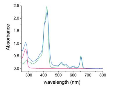
**Figure 1.** UV-Vis spectra of mTHPC@HSA (blue line) in PBS, HSA (magenta line) in PBS, and mTHPC in DMSO (green line).
