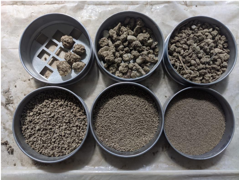
236 Fig. 4. From left to right and top to bottom: Sieves with diameters d_i of 31.5, 16, 8, 4, and 2 237 mm and the residual collector.
