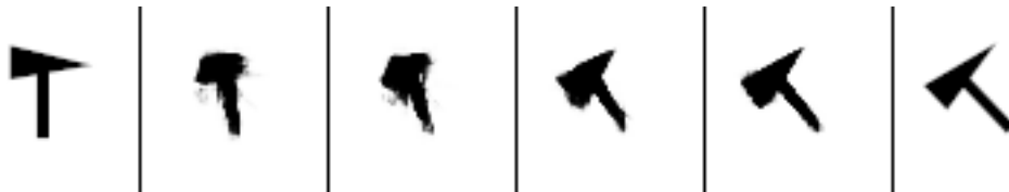
FIGURE 2. Reconstruction of missing images in the case of the hammer shape, with the parameters D = 64 , h_1 = 0.7 , h_2 = 5 , N_{\text{iter}} = 1000 and \varepsilon = 0.04 . We also processed the image applying a smooth threshold via the \Sigma sigmoid function.
