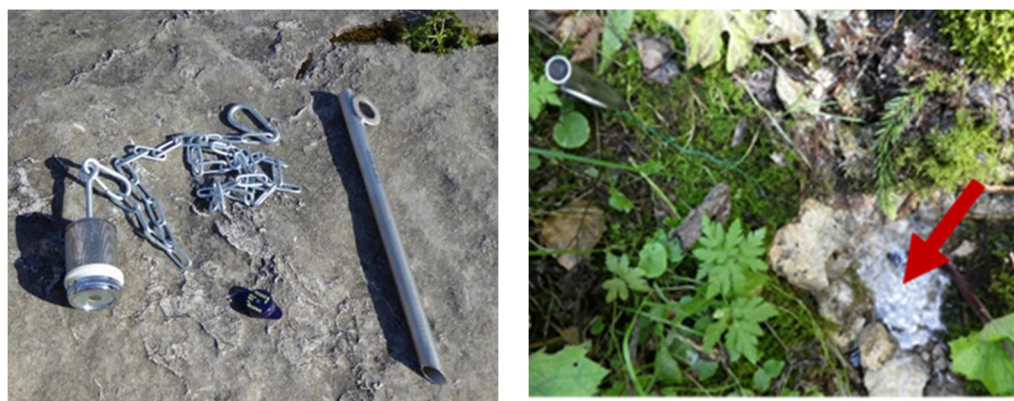
Figure 5. Metal rod, chain and metal basket to fix and protect the data logger against bed load (left). Attachment of a data logger in a spring (right).
