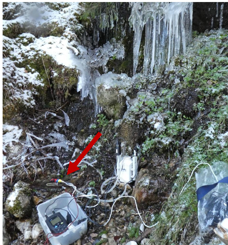
Figure 4. Application of a flow pump (marked by the red arrow) during winter low-discharge conditions in the field in the Berchtesgaden National Park to keep measuring sensors constantly covered with water.
