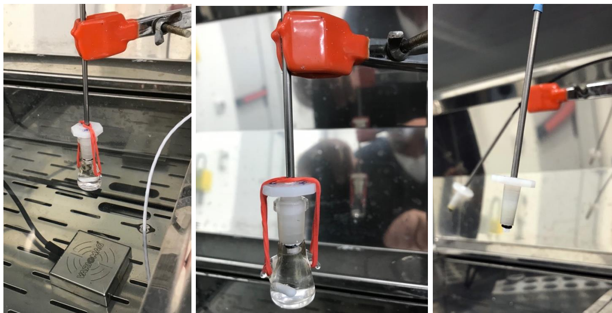
Figure S1. Scheme of the real-time oxygen sensing equipment (top) and images of the assembly of sample vials (int. volume 2.4 mL) with the oxygen probe sealed through the cap (bottom).
