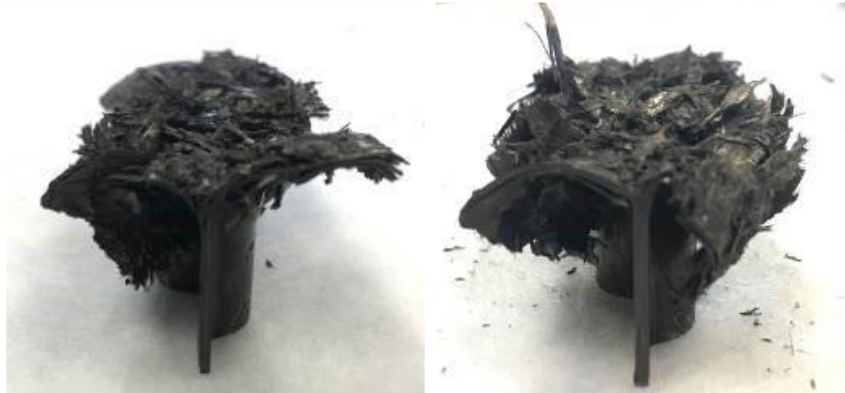
Figure 20. Example of lateral ply splaying for [0]_6 layup (left) and [45/0]_s layup (right).
