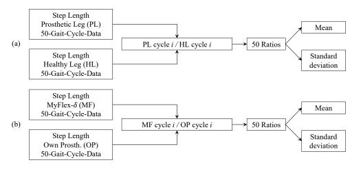
**Figure 15.** Procedures for the calculation of: (a) the ratio between the step length measured from the prosthetic leg and the healthy leg; (b) the ratio between the step length measured while using MyFlex- $\delta$  and while using a participant's own prosthesis.
