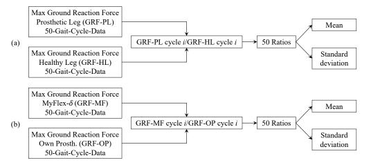
**Figure 10.** Procedures for the calculation of: (**a**) the ratio between the ground reaction force measured from the prosthetic leg (GRF-PL) and the healthy leg (GRF-HL); (**b**) the ratio between the ground reaction force measured while using MyFlex- $\delta$  (GRF-MF) and while using their own prosthesis (GRF-OP).
