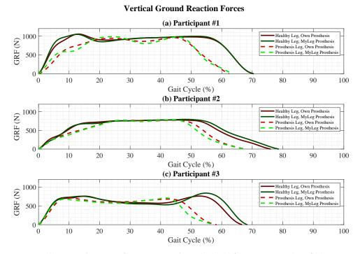
**Figure 9.** The ground reaction forces mean value calculated from 50 gait cycles of (a) Participant 1, (b) Participant 2 and (c) Participant 3: healthy leg, using their own prosthesis (dark red straight line); healthy leg, using MyFlex- $\delta$  (dark green straight line); prosthetic leg, using their own prosthesis (light red dashed line); prosthetic leg, using MyFlex- $\delta$  (light green dashed line).
