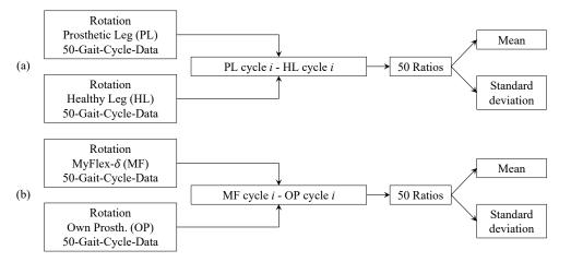
**Figure 12.** Procedures for the calculation of: (**a**) the difference between the rotation measured from the prosthetic leg and the healthy leg; (**b**) the difference between the rotation measured while using MyFlex- $\delta$  and while using their own prosthesis.
