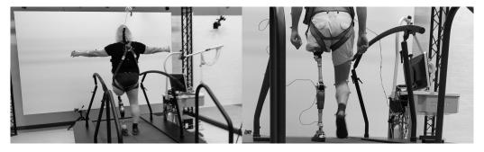
**Figure 5.** Treadmill test: the participant's movements are measured thanks to the reflective markers placed on their skin. The participant wore a harness for safety.
